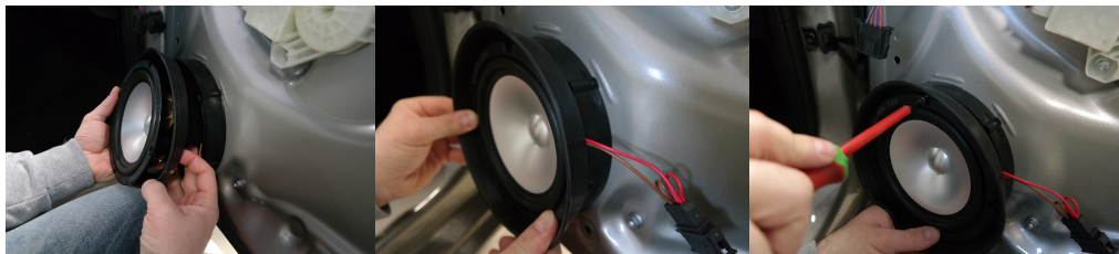
Step 2: Positioning of the midwoofer with the sealing ring and fastening using the included screws (4.2x19mm)
