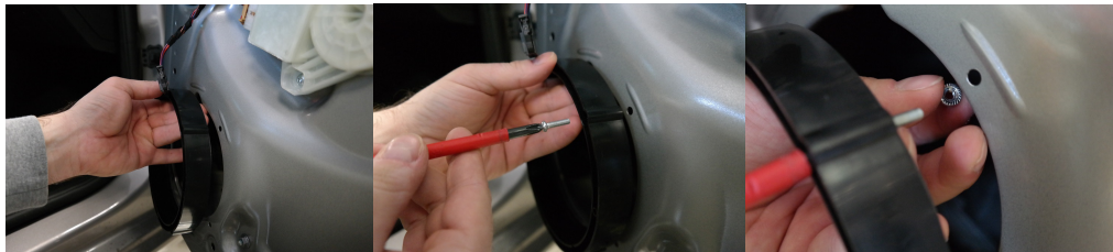
Step 1: Positioning of the spacer and fastening using the included metric bolts and nuts
