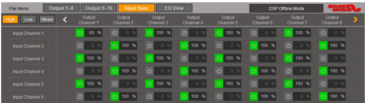
Figure 2 shows that the audio signal of output channel 1 comes from input channel 1,3,5 mixed. Similarly, output channel 2 comes from input channel 2,4,6 mixed, output channel 3 comes from input channel 1,3,5 mixed.....
