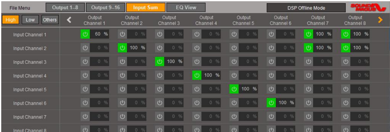
Figure 2 shows that the audio signal of output channel 1 comes from input channel 1,3,5 mixed. Similarly, output channel 2 comes from input channel 2,4,6 mixed, output channel 3 comes from input channel 1,3,5 mixed.....
